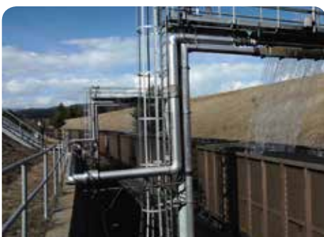
Rail cars carrying coal are covered with a coating to keep the coal in the rail cars while in transit.
