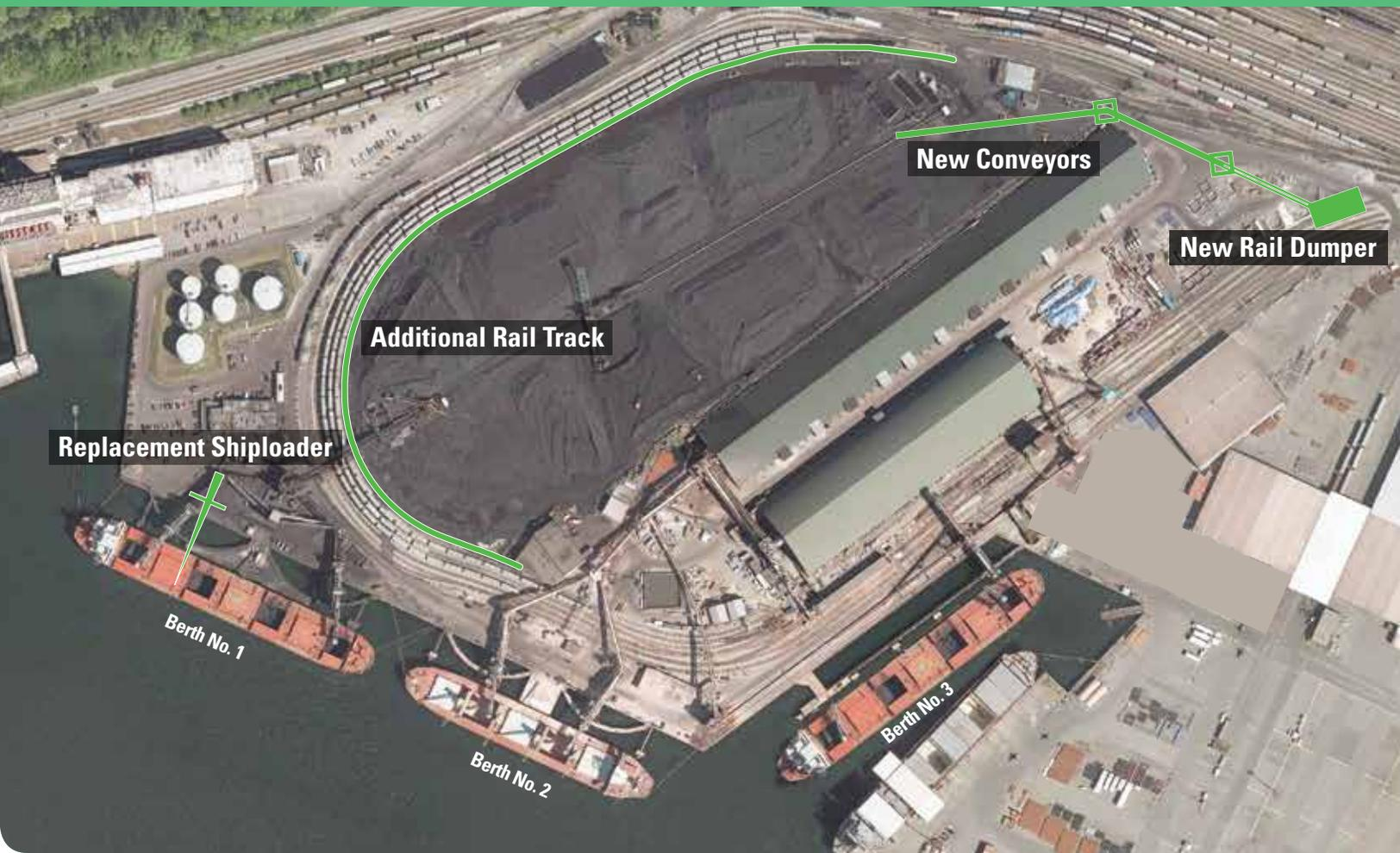
An aerial view of Neptune's site showing the planned new conveyors, second railcar dumper, additional rail track and replacement shiploader.
