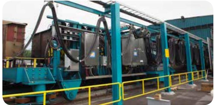
Neptune's automated electric indexer is used for positioning railcars, as an alternative to locomotives.
