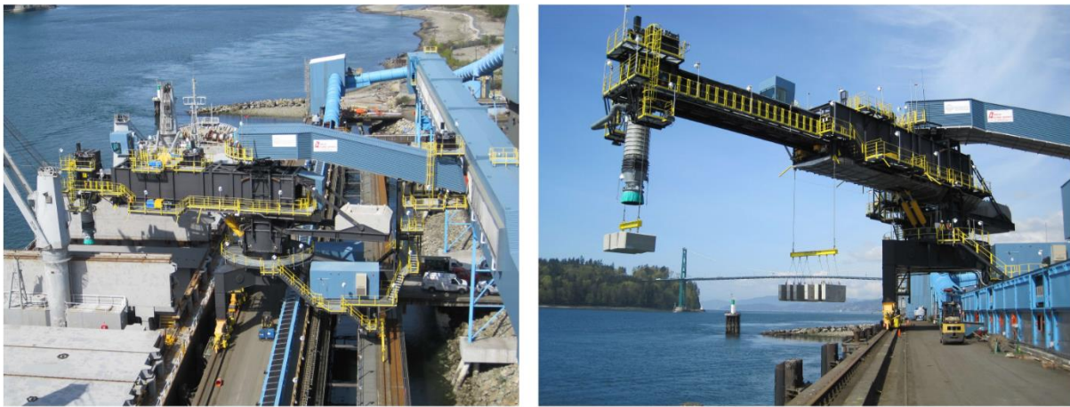
Figure A- 2: New Traveling Slewing Potash Shiploader (reference photo from similar facility)
